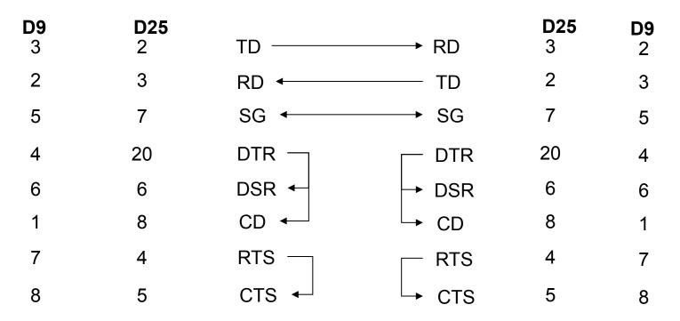
Full-duplex connection between two DTEs. No flow control necessary since both DTEs send at the same speed.
